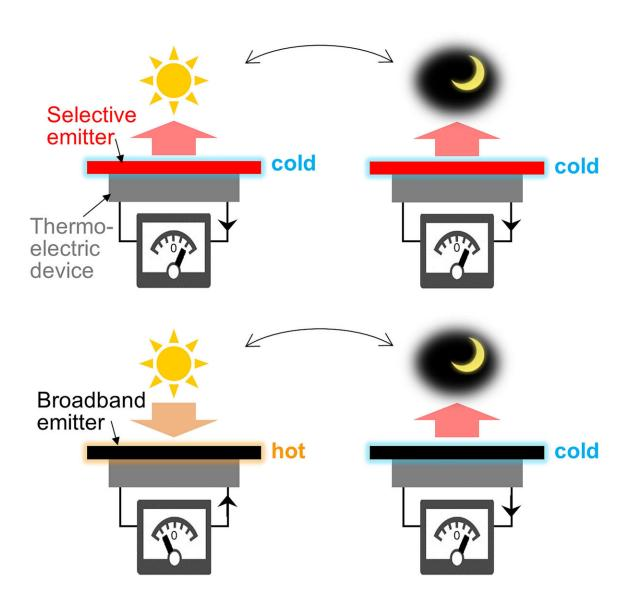
An illustration of thermoelectric devices using a wavelength-selective emitter and a broadband emitter. The device using a broadband emitter experiences a
