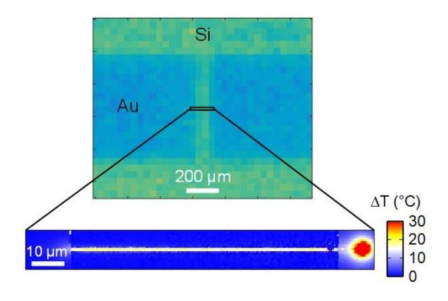
Temperature map of a gold nanowire on a silicon substrate, Joule-heated by the application of an electrical current of 7 mA, obtained through infrared thermography (top) and a spin-crossover surface thermometer (bottom). While heating remains undetectable in infrared due to low thermal and spatial resolution, temperature distribution is well resolved using an SCO-based thermometer, which reveals a "hot spot" resulting from a malfunction of the component. Credit: Ridier et al.
