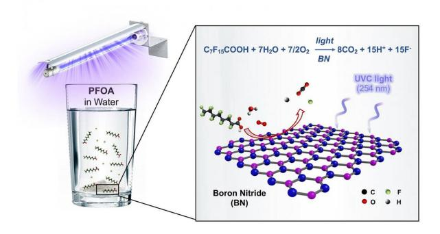
An illustration of the boron nitride photocatalysis that destroys the pollutant PFOA in water. Credit: Image courtesy of M. Wong/Rice University
