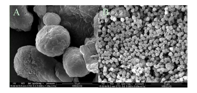
SEM images of polyethylene (PE) (A) and polyvinyl chloride (PVC) particles (B). Credit: WBG
