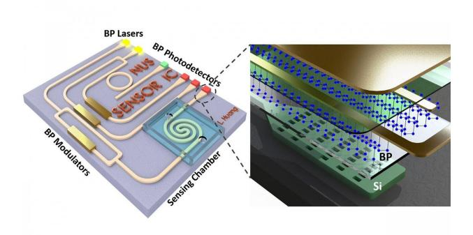
Schematics of an on-chip mid-infrared system based on black phosphorus-silicon hybrid platform. The passive silicon photonic layer serves to guide the midinfrared light while black phosphorus plays an active role in light emission, modulation and detection. Credit: Bowei Dong and Li Huang
