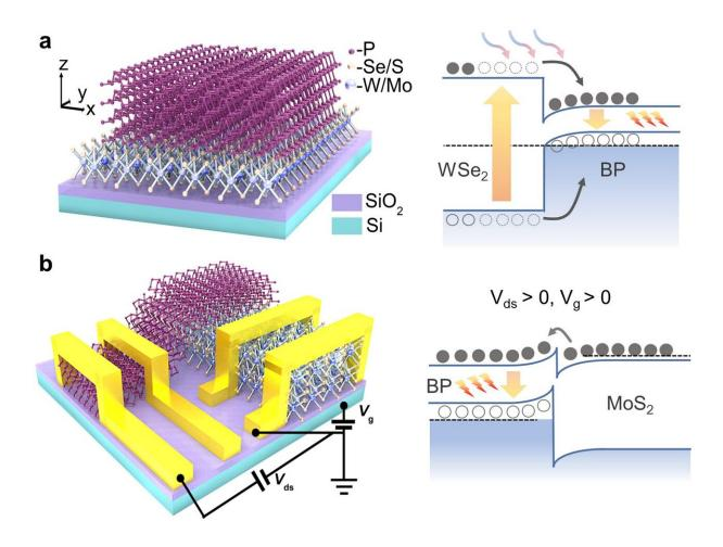
a, Schematic diagram of the BP-WSe2 heterostructure. Under the excitation of light, the electron and hole pairs in WSe2 can be efficiently transmitted to BP, thereby enhancing its MIR photoluminescence. b, Schematic diagram of the BP-MoS2 heterojunction diode. Under a positive bias voltage between BP and
