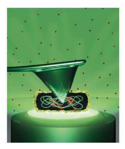
Simultaneous AFM nanoindentation and fluorescence imaging of E. coli. Credit: Patricia Bondía
