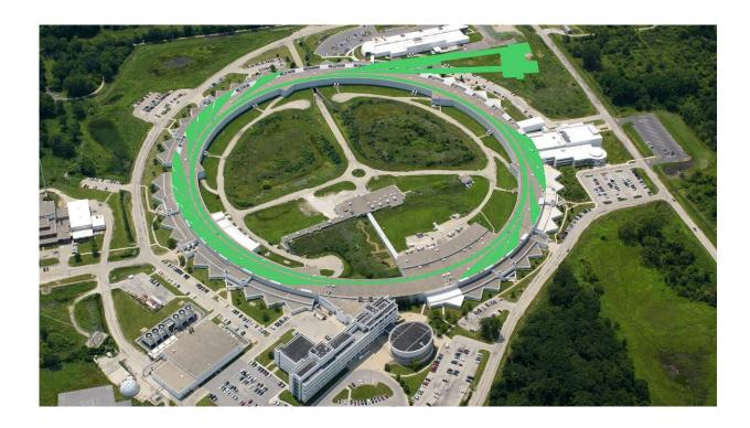
This superimposed image shows the storage ring and beamlines that will be newly built or updated for the APS Upgrade, including the Long Beamline Building (upper right), a new structure that will house two longer beamlines. Credit: Mark Lopez / Argonne National Laboratory
