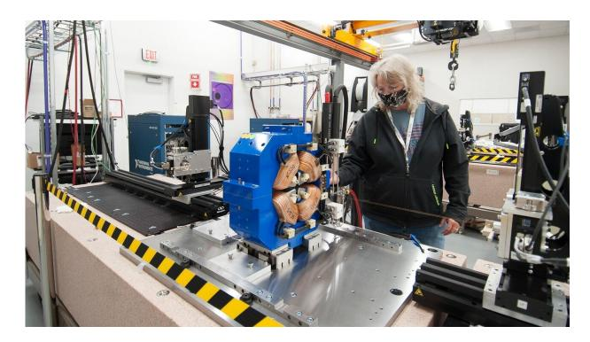
Kris Meitsner of the APS Engineering Support division Survey and Alignment group tests a quadrupole magnet at Building 369 for installation as part of the APS-U. Credit: Rick Fenner / Argonne National Laboratory
