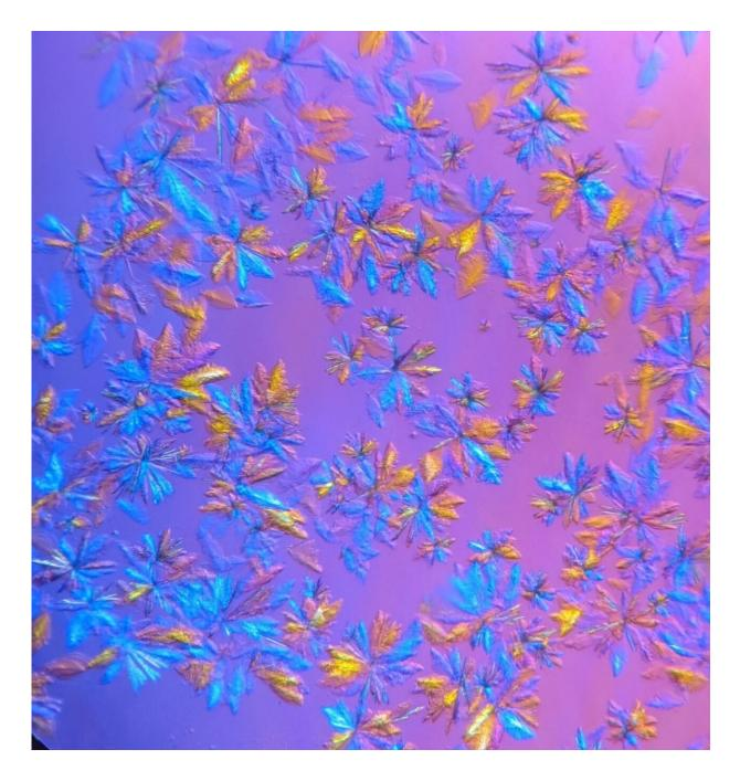
SARS-CoV-2 protease crystals, grown in ORNL's Protein Crystallization and Characterization laboratory and pictured in microscopic view, will be used in Xray scattering experiments. Credit: Daniel Kneller/ORNL, U.S. Dept. of Energy
