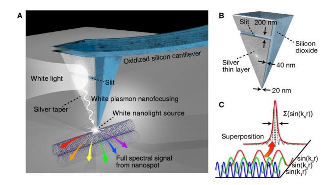
Plasmon nanofocusing of white light for full spectral nanoanalysis. (A)Schematic of plasmon nanofocusing for white light and spectral bandgapnanoanalysis. (B) Schematic of tapered metallic structure used for simulation.(C) Superposition of waves with different wave vectors. Credit: ScienceAdvances, doi: 10.1126/sciadv.aba4179
