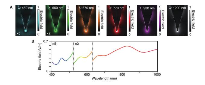
Broadband property of plasmon nanofocusing evaluated by FDTD simulations. (A) Electric field distribution maps in the vicinity of the apex of the tapered silver structure produced by FDTD simulations. Scale bars, 100 nm. The plasmon coupler slit, where white light was illuminated, is not shown, as it is out of the frame. (B) Simulated near-field spectrum detected 6 nm below the apex. Credit: Science Advances, doi: 10.1126/sciadv.aba4179
