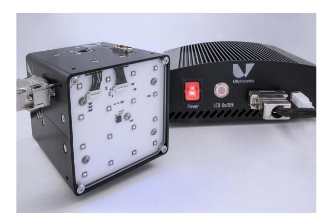
Modular LED irradiation system equipped with UVC LEDs for disinfection. Credit: FBH/P. Immerz
