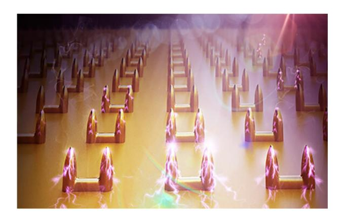
An illustration of a 3-D metasurface trapping light with extremely strong nearfield enhancement at the tips of pillars through dark modes. Credit: Swinburne University of Technology
