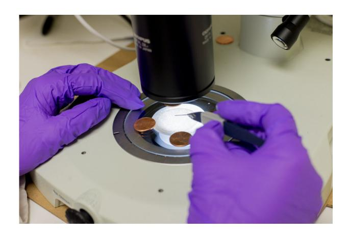
Researchers examined filters from field sites in several national parks and wilderness areas and did visual counts of microplastic beads and fragments deposited by wind and precipitation. The pennies are used to hold each filter in place on the microscope stage. Credit: Brian Kartchner, Utah State University
