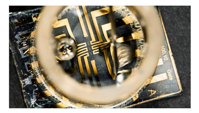
The organic electrochemical transistor in which the researchers have been able to deposit Shewanella oneidensis on one of the microelectrodes. Credit: Thor Balkhed
