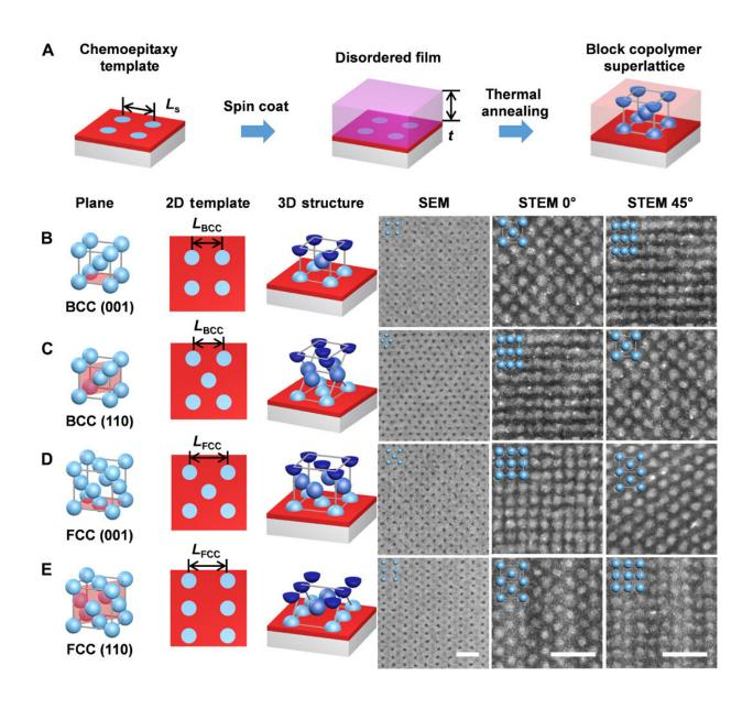
Controlling the symmetry and orientation of a BCP superlattice. (A) Schematic
