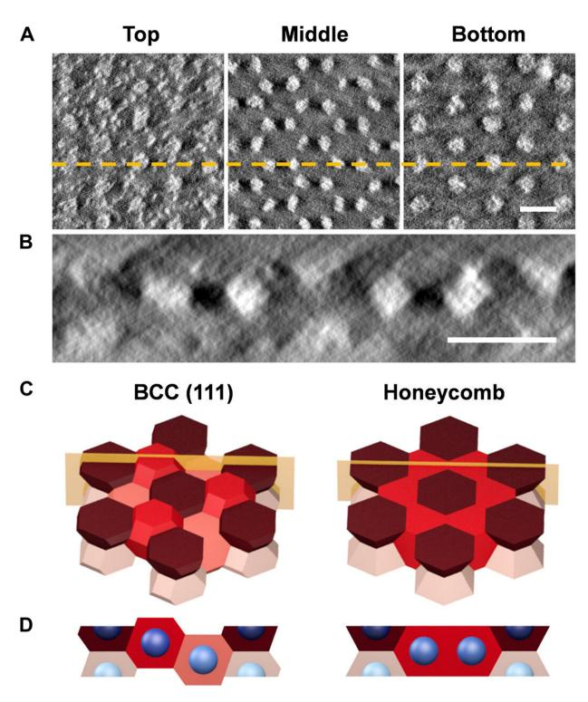
Formation of honeycomb lattice through lattice distortion. (A) In-plane slices created from STEM tomography showing the hexagonal symmetries at the top and bottom layers and the honeycomb symmetry in the middle layer. (B) Digitally sliced cross-section along the golden dashed line in (A) showing the
