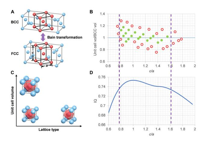
Bain transformation with 3D DSA. (A) BCC and FCC lattices can be connected
