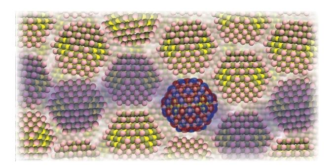
Tightly packed crystals in a nanocrystal semiconductor: the model developed by ETH researchers describes every single atom. Credit: ETH Zurich / Nature Communications
