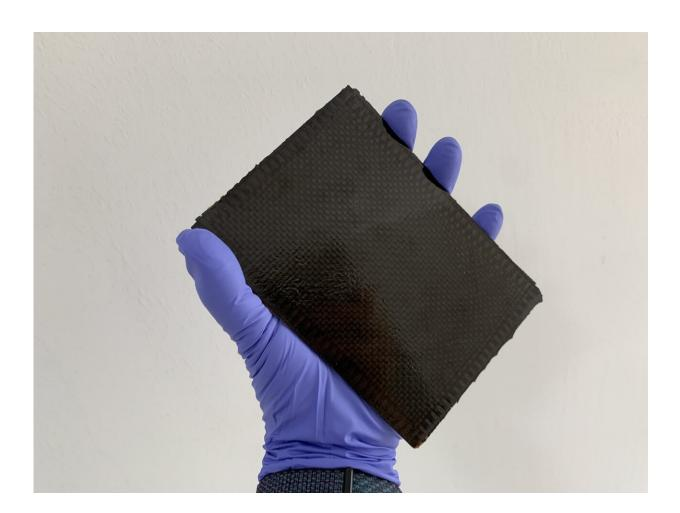
KIST research team used plant-originated tannic acid to develop a flameretardant carbon fiber-reinforced plastic (CFRP) Credit: Korea Institute of Science and Technology
