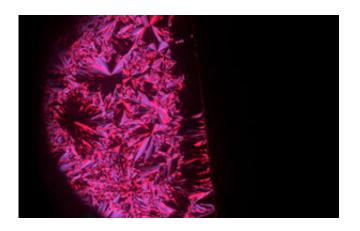
A polarized optical microscopy image of the columnar liquid crystals sandwiched between two crossed polarizers with (right) and without (left) an electric field. This suggests that applying an electric field breaks the symmetry of the liquid crystals. Credit: American Chemical Society
