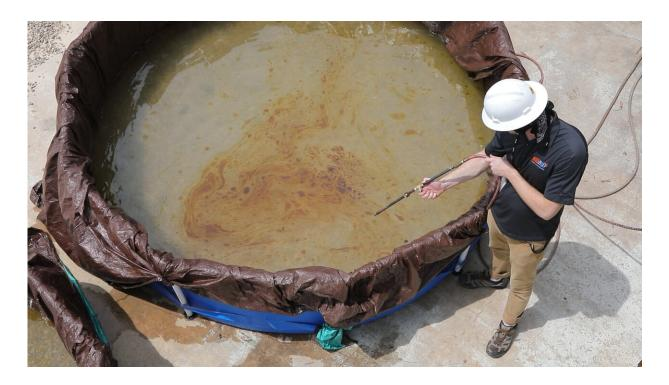
SwRI engineers added two types of oil to tanks of water to train cameraequipped machine learning algorithms to detect oil under various lighting and environmental conditions. Credit: Southwest Research Institute
