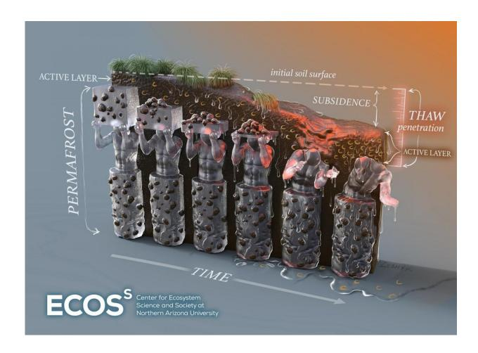
A time series shows ground-ice 'atlases' in permafrost struggling to support the active layer as soil temperatures warm and accelerate thaw. As ice is lost, we see a significant shift in the soil surface over time, and the need to account for subsidence in measurements. Credit: Victor Leshyk, Center for Ecosystem Science and Society
