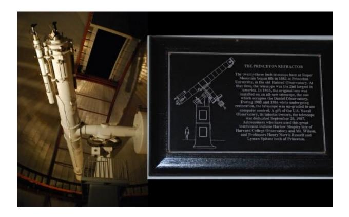
The 23" Princeton refractor, with the 5" finder used for the 1906 Venus observation clearly seen. This telescope is now installed at the Roper Mountian observatory in South Carolina. Credit: Dave Dickinson
