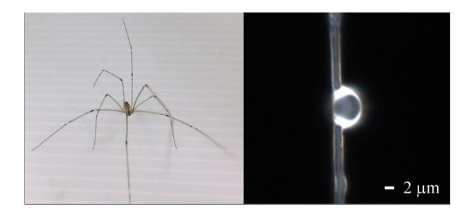
An image of the spider used in the study and the dome lens generated on its dragline silk. Credit: Cheng-Yang Liu
