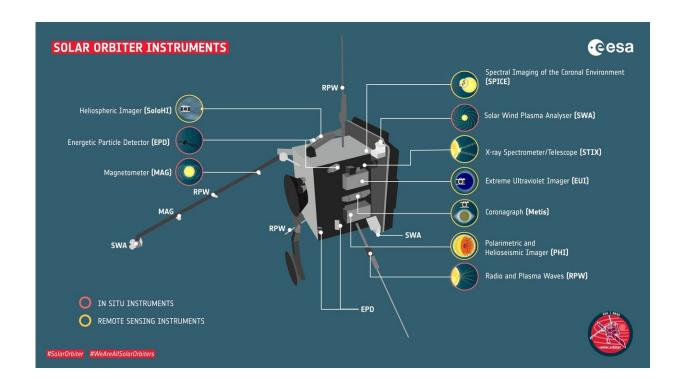
Solar Orbiter instruments, Credit: ESA-S.Poletti
