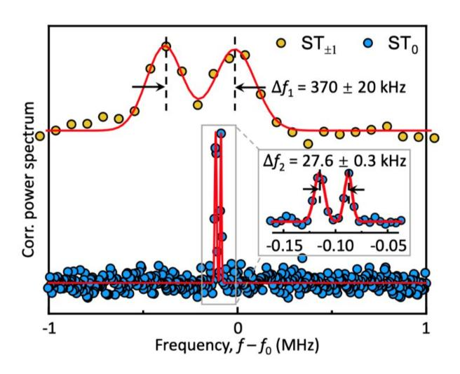
The comparison of the paramagnetic resonance spectrum between the traditional method (top) and the new method (bottom) of noise-insensitive. It clearly shows that the spectral resolution has been significantly improved, and more precise coupling information has been observed. Credit: DU Jiangfeng et al.
