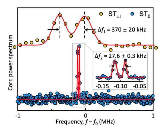
The comparison of the paramagnetic resonance spectrum between the traditional method (top) and the new method (bottom) of noise-insensitive. It clearly shows that the spectral resolution has been significantly improved, and more precise coupling information has been observed. Credit: DU Jiangfeng et al.
