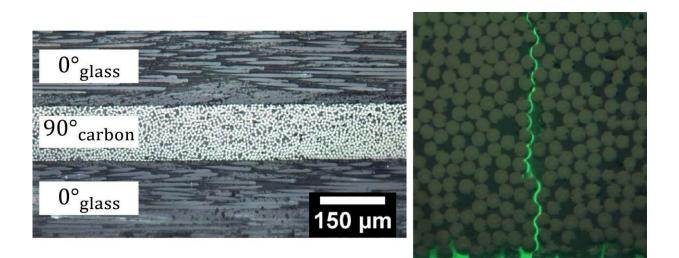
Optical image of a composite laminate used in the transverse failure experiments. Right: Representative image of a transverse crack spanning the 90 ply. As apparent from this optical image, the transverse cracks extend primarily along fiber/matrix interfaces. Credit: University of Illinois Dept. of Aerospace Engineering
