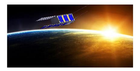
Led by the Royal Meteorological Institute Belgium, Simba is a 3-unit CubeSat mission to measure the Total Solar Irradiance and Earth Radiation Budget climate variables with a miniaturised radiometer instrument, due to be launched in 2020 on the inaugural flight of the ESA's developed 'Small Spacecraft Mission System' dispenser – devoted to CubeSats and other small satellites – on a Vega launcher. Credit: RMI
