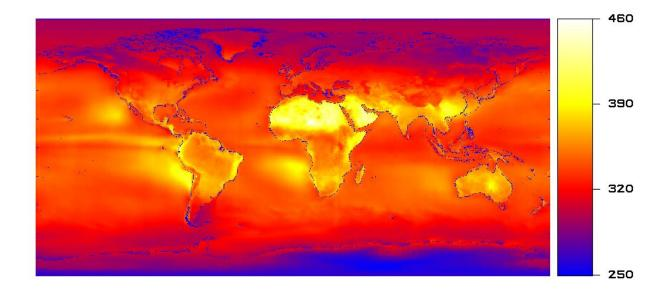
Simulated results from the Simba CubeSat mission, which will employ a radiometer to measure solar irradiance levels across Earth's surface to help study meteorology and climate change. Credit: European Space Agency
