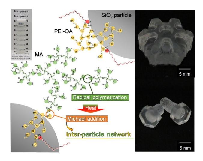
Interparticle photo-cross-linkable suspension enables 3D structuring of transparent SiO2 glass components through rapid heating profiles. Credit: Motoyuki Iijima, Yokohama National University
