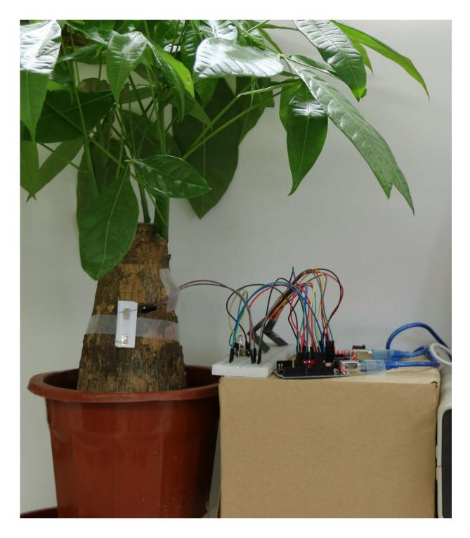
A sensor (white strip) on a houseplant activates an alarm when fire is near. Credit: Adapted from ACS Applied Materials & Interfaces 2020
