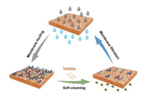
Schematic diagram of N-TiO<sub>2</sub> and TiO<sub>2</sub> coated membrane preparation and mechanism of visible-light-activated photocatalysis for fouling mitigation. Credit: ZHANG Huiru
