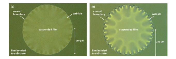
Wrinkling in the diamond window is caused by stress in the layers of diamond and glass. The diamond window in image a, which is smaller than the diamond window in image b, has a higher density of wrinkles. Credit: Okinawa Institute of Science and Technology
