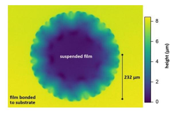
The scientists used a laser microscope to determine the height across the surface of the diamond window in order to calculate the level of strain. For this diamond window, the suspended nanocrystalline diamond film buckles downwards below the glass surface. Credit: Okinawa Institute of Science and Technology
