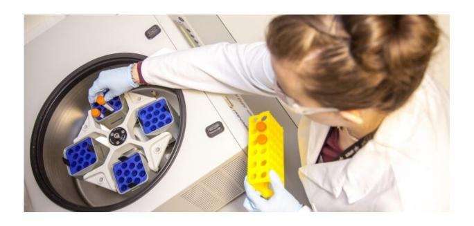
Samples being placed into a centrifuge to separate sample components. Credit: Swansea University
