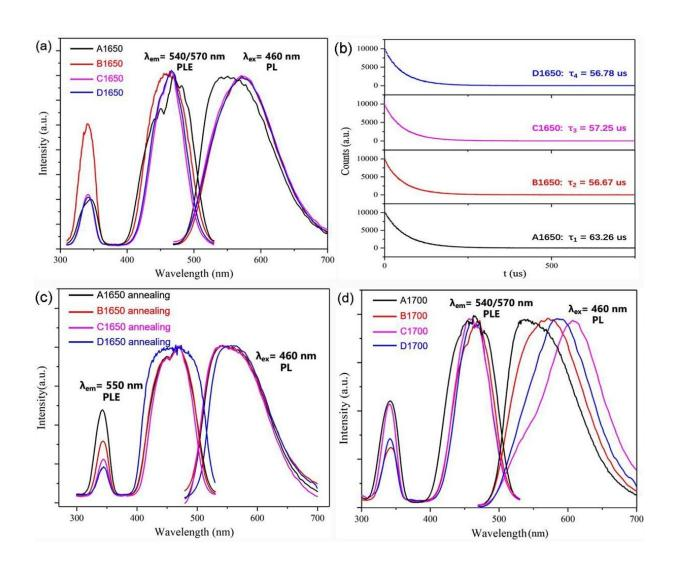
(a) The PL and PLE spectra of A1650-D1650; (b) The luminescence decay profile of A1650-D1650; (c) The PL and PLE spectra of A1650-D1650 after annealing in the air; (d) The PL and PLE spectra of A1700-D1700. Credit: SIOM
