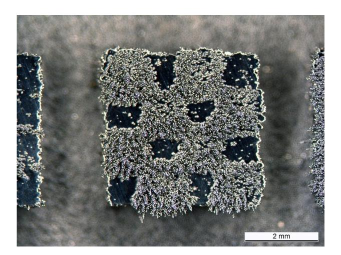
Empa Precisely Magnetized: Iron filings stick to this mini chessboard with four millimeter edge length. The partially magnetic structure was produces from a single type of steel power at different temperatures. Credit: Swiss Federal Laboratories for Materials Science and Technology
