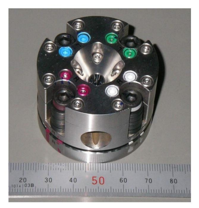
A metal sample is placed inside a rhenium gasket with thermal insulators, squeezed between two diamonds to generate high pressure, and heated with a near-infrared laser. Density measurements under such high-pressure and high-temperature conditions are made by irradiating the sample with x-ray beams. Credit: Assistant Professor Yoichi Nakajima
