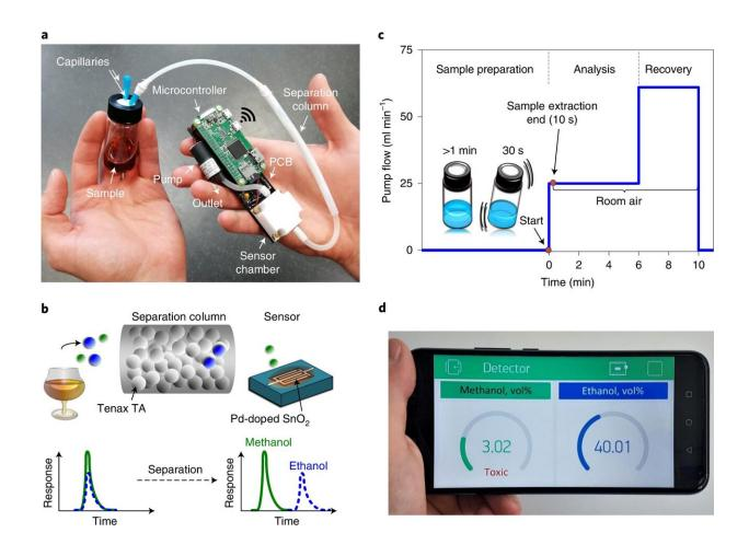
Analyser design. a, The handheld analyser during measurement. b, A schematic of the detection concept. c, The sampling and analysis procedure. d, The tailor-made app to visualize results on a smartphone transmitted through a wireless local area network. PCB, printed circuit board; Pd, palladium. Credit: *Nature Food* (2020). DOI: 10.1038/s43016-020-0095-9
