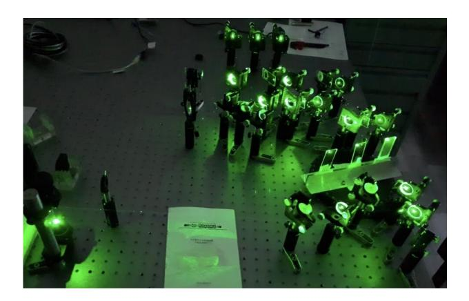
Apparatus for measuring the position of an object using optical coherence alone. Credit: Nikita Kirsanov/MIPT
