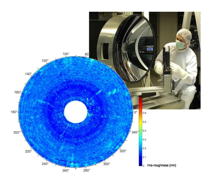
Light scattering based surface characterization of a substrate for EUV lithography. Credit: Fraunhofer IOF
