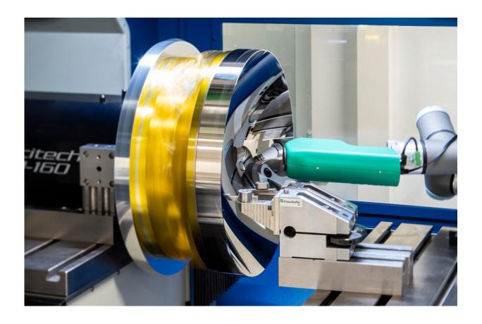
Roughness inspection during diamond turning with a light scattering sensor. Credit: Fraunhofer IOF
