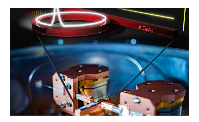
Experimental setup to generate a set of stable frequencies in a cryogenically cooled laser microresonator frequency comb. The ring-shaped microresonator, small enough to fit on a microchip, operates at very low laser power and is made from the semiconductor aluminum gallium arsenide. Credit: NIST
