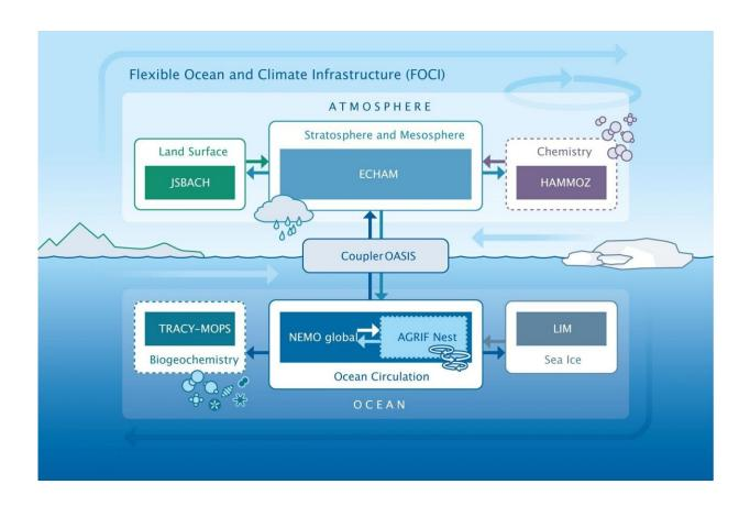
Schematic Diagram of the FOCI Model System with the difference components Credit: C. Kersten, GEOMAR
