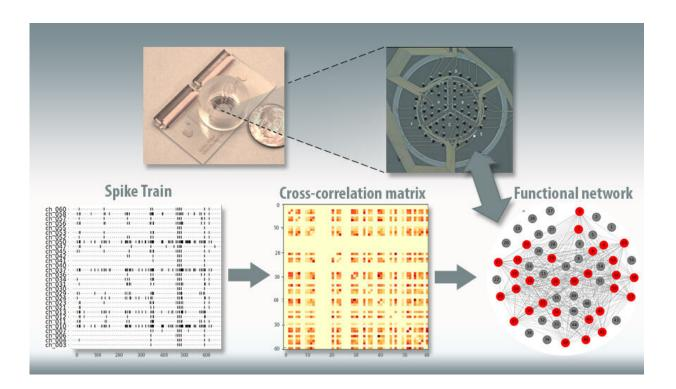
This figure depicts Lawrence Livermore National Laboratory's "brain-on-a-chip" device (top). Electrical recordings from the chip (lower left), taken from seeded neurons, are used to model correlations between electrodes (center), and these correlations are used to create a model of the network structure in the chip (lower right). Credit: Lawrence Livermore National Laboratory
