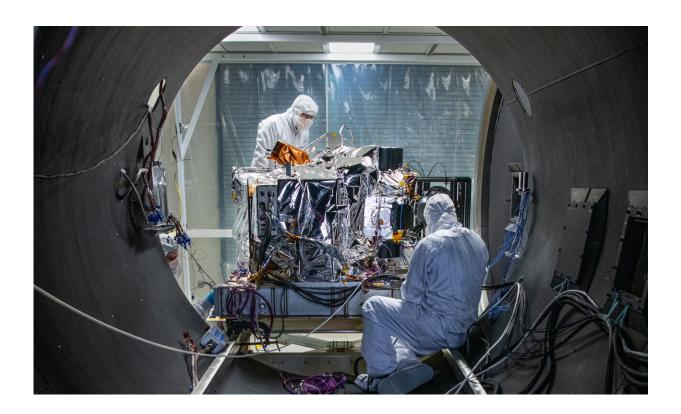
After passing its last critical design review in February, PACE has entered its integration and testing phase of development. A mockup of the Ocean Color Instrument is under construction at NASA's Goddard Space Flight Center in Greenbelt, Maryland, and both the instrument and spacecraft will soon be tested in rigorous conditions that simulate launch and orbit. Credit: NASA / Dennis Henry
