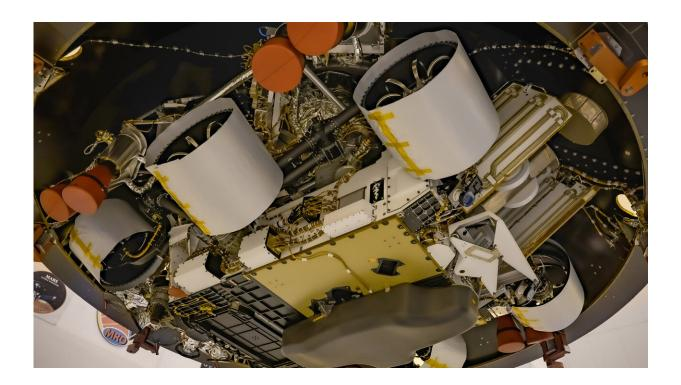
This photo provided by NASA/JPL-Caltech in June 2020 shows a 3-by-5-inch (8-by-13-centimeter) aluminum plate between the wheels at center and right, which commemorates the impact of the COVID-19 pandemic and pays tribute to the perseverance of healthcare workers around the world, attached to the Perseverance Mars rover, in Pasadena, Calif. NASA is pressing ahead with a July 20 launch, despite the pandemic. (NASA/JPL-Caltech via AP)
