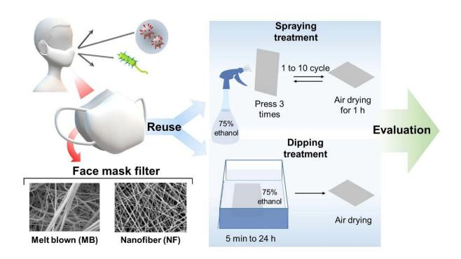
Schematic diagram on spraying and dipping treatments of face mask filters. Credit: ©2020 American Chemical Society
