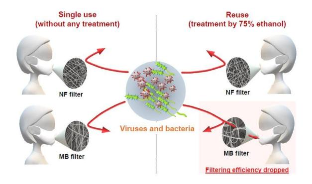
Comparison of mask filter performance after ethanol disinfection: The nanofiber filter has air permeability even after being washed. The melt-blown filter has its mesh structure changed by ethanol sterilization and its performance is deteriorated. Credit: © 2020 American Chemical Society
