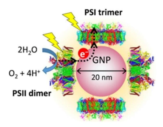
Schematic view of a PSI-GNP-PSII conjugate designed in this study. The electron acceptor and donor sides of PSII and PSI complexes, respectively, are attached to a GNP through (His)6 tags and Ni-nitrilotriacetic acid (Ni-NTA), and thus electrons abstracted from H2O in PSII are expected to be transferred to PSI upon illumination. Credit: IOS Press
