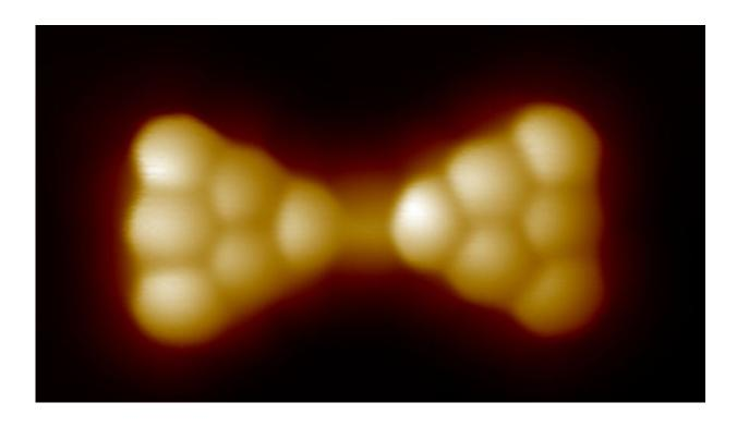
When graphene nanotriangles are joined, their magnetic moments form a "quantum entangled" state. Credit: Empa
