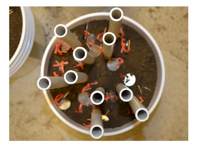
The assembled loamy soil experimental buckets at the beginning of the experiment. PVC tubes with rust paint and wooden sticks were used to track oxygen and decomposition. Credit: M.C. Rabenhorst
