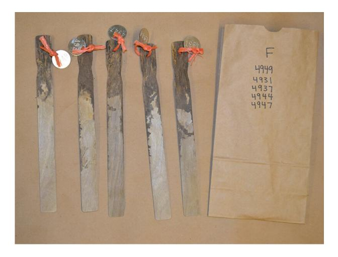
The wooden birch sticks after being in the capillary fringe experimental buckets for 118 days. The sticks were taken out of the soil, rinsed, dried, and weighed to determine how much decomposition had occurred. Credit: J.C. Fiola
