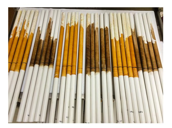
PVC pipes painted with rust, known as IRIS tubes, help track how much oxygen is in the soil. When there isn't enough oxygen, microbes will turn the rust into regular iron, which washes away. These tubes are drying after being extracted from the experiments and rinsed. Credit: J.C. Fiola
