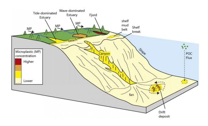
Shelf and deep sea environments have generally lower micropastic flux rates than coastal environments, but high rates may occur locally where bottom currents concentrate microplastic (e.g. on drift deposits, in submarine canyons and ocean trenches; Kane et al., 2020) or beneath locations of high particulate organic carbon flux driven by primary production (Tekman et al., 2020). Credit: Peter T. Harris, https://doi.org/10.1016/j.marpolbul.2020.111398
