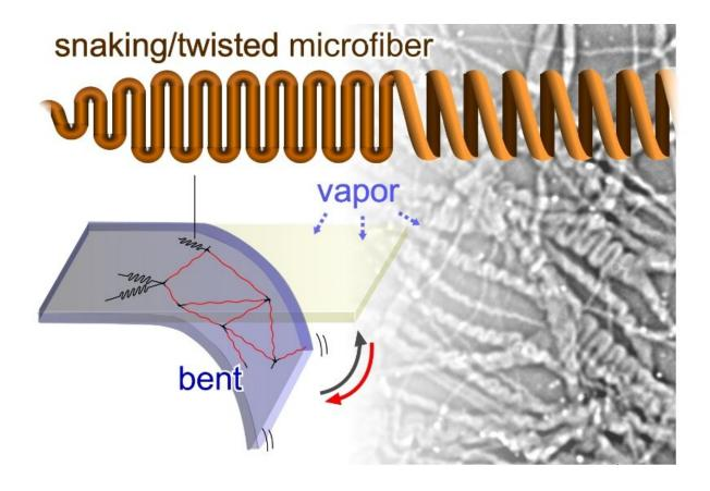
Schematic illustration of the humido-sensitive film composed of a snaking/twisted fiber network. Credit: JAIST
