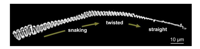
Optical microscopy image of a single fiber of self-assembled polysaccharide in snaking, twisted, and straight structures. Credit: JAIST
