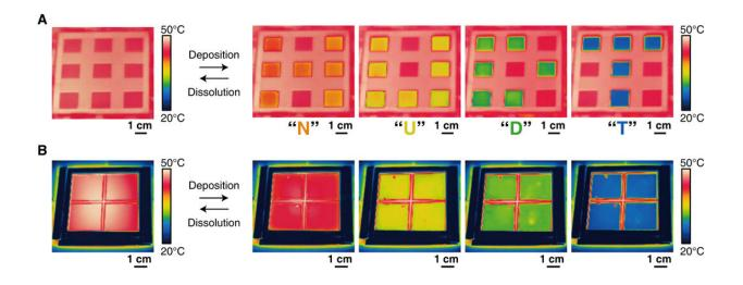
Multiplexed and enlarged adaptive devices. (A) LWIR images of a three-bythree multiplexed array (left) before and (right) after selective electrodeposition of different pixels for different times. (B) LWIR images of an enlarged independent device (left) before and (right) after electrodeposition for different times. Photo credit: Mingyang Li, National University of Defense Technology. Credit: Science Advances, doi: 10.1126/sciadv.aba3494
