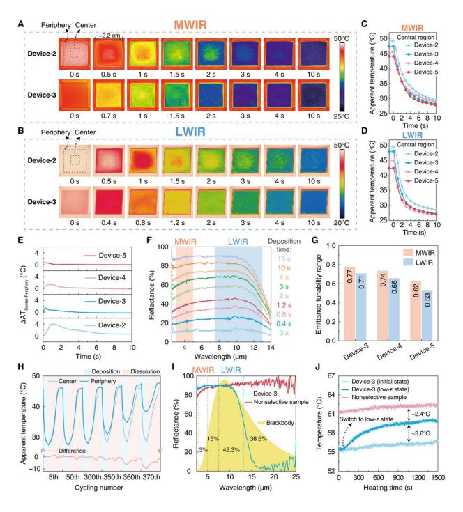
Dynamic IR performance. (A and B) Real-time MWIR and LWIR images of device-2 and device-3 during the electrodeposition process, respectively. (C and D) Apparent temperature curves (central region) of the assembled devices in the MWIR and LWIR images during the electrodeposition process. (E) Apparent temperature difference curves between the central and peripheral regions of the assembled devices in the LWIR images during the electrodeposition process. (F)
