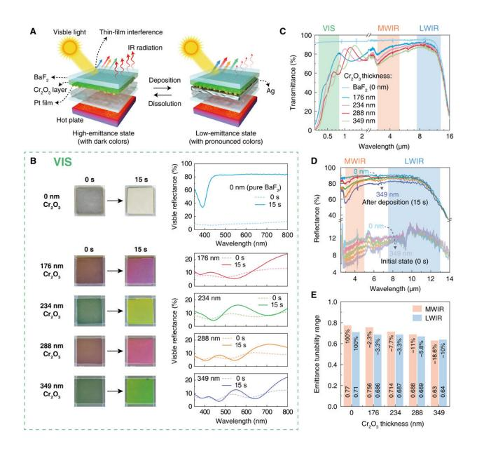
Visible compatibility. (A) Schematics of a visible-wavelength-scale-thick Cr2O3 layer decorated adaptive device (left) before and (right) after electrodeposition.(B) Photographs and "real-time" visible reflectance spectra of the Cr2O3
