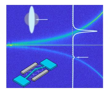
"Satellites" in the spectrum of a vibrating nanostring (lower image insert) for increasing drive power. The different brightnesses of the upper (green) and lower (blue) satellite encode the strength of the squeezing (upper image insert). Credit: Weig group
